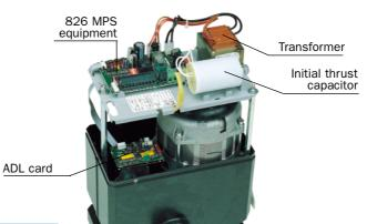
Enbloc base in pressure cast aluminium, with cataphoresis treatment
